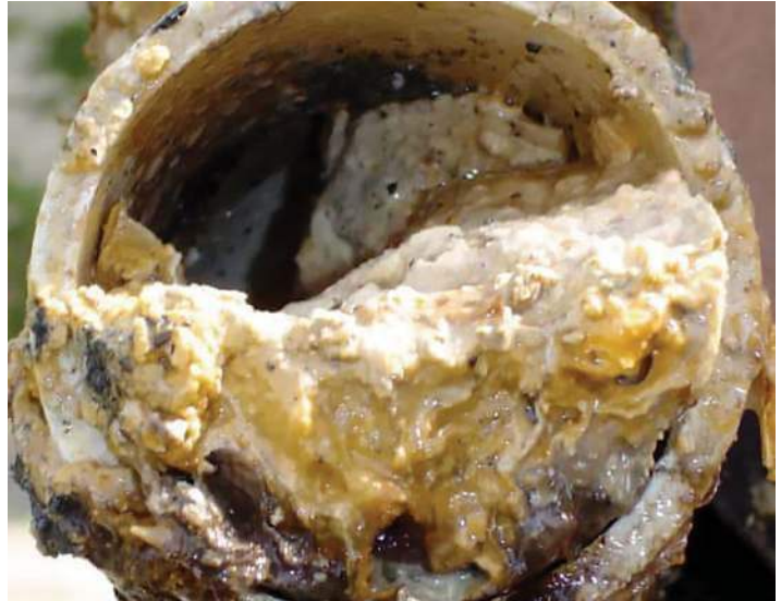
Fatbergs – fats, oils, and grease combined with solids – can clog sewer systems. (Contributed photo)
