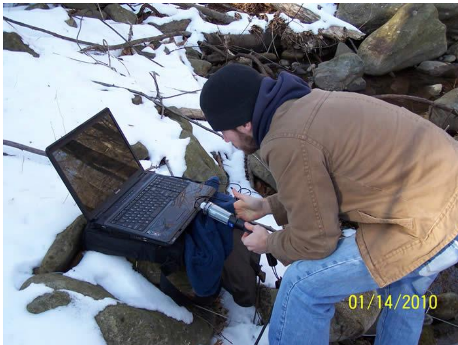
Researcher Scott Collenberg shown downloading data from a HOBO logger to his laptop.
